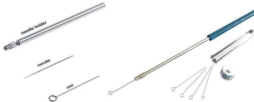
Gambar 32. Jarum inokulum (jarum ose dan *inoculating needle*)
